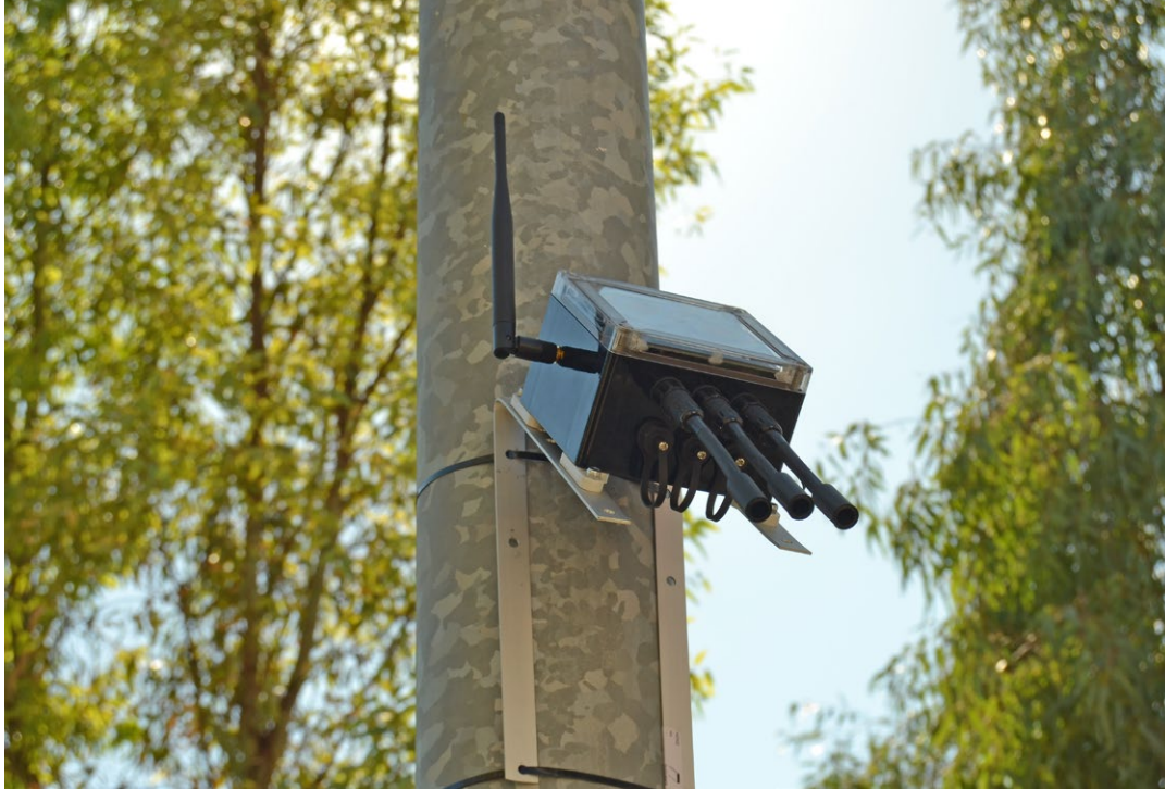
Figure 4: Waspote Plug & Sense! powered by an internal solar panel
