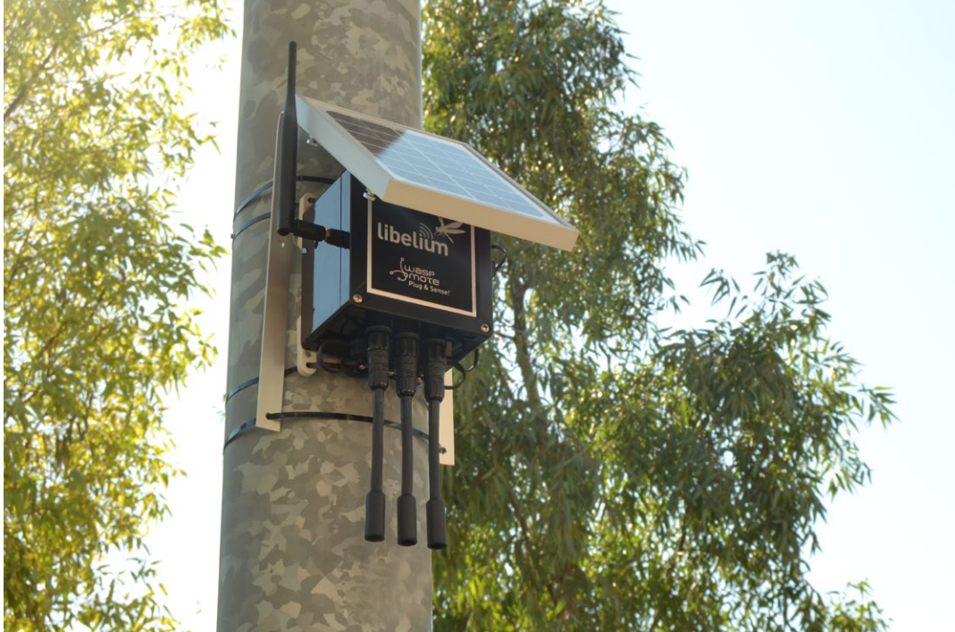
Figure 2: Waspote Plug & Sense! powered by an external solar panel
